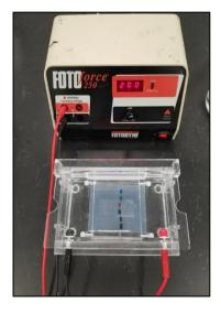
*Gel box connected to power supply*
