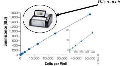
The figure above shows both a luminometer and the sort of data generated by measuring light. The data shows that the more living cells that are present in the sample, the greater amount of luminescence, measured in **R**elative Light Units (**RLUs**), that is produced by those cells. The light produced in this experiment is not bright enough to see with the naked eye, so it must be measured using a luminometer.
